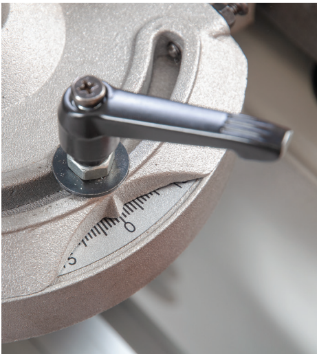
Fence mitre scale, pointer and clamping handle
