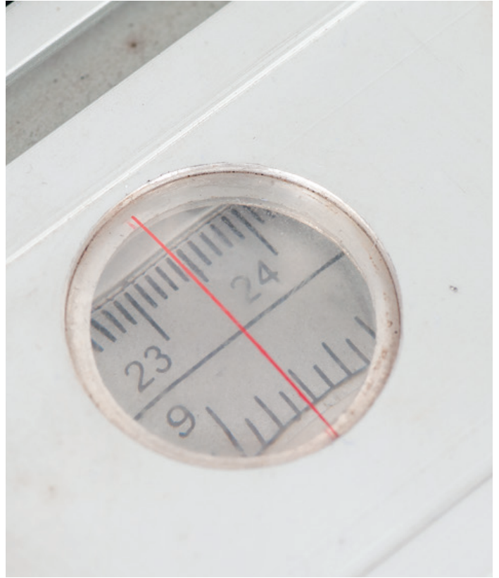
Rip fence magnifying glass and index marker
