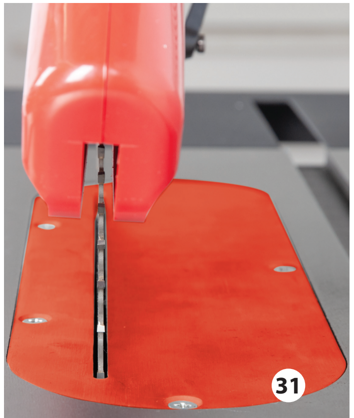
Optional 104933 insert gives better material support for cutting thin strips
